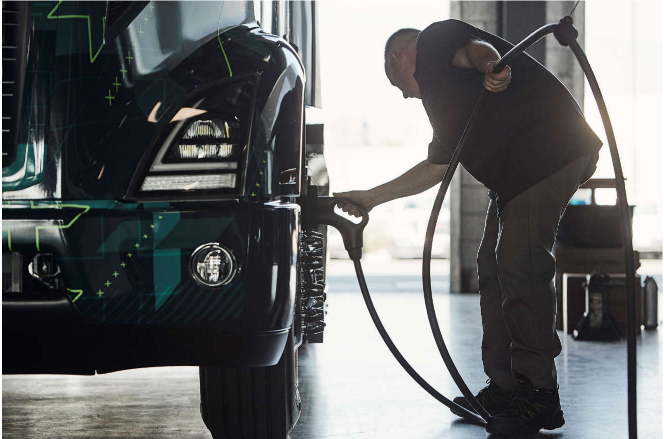
Figure 4. A Volvo VNR Electric is being plugged in to charge up.
