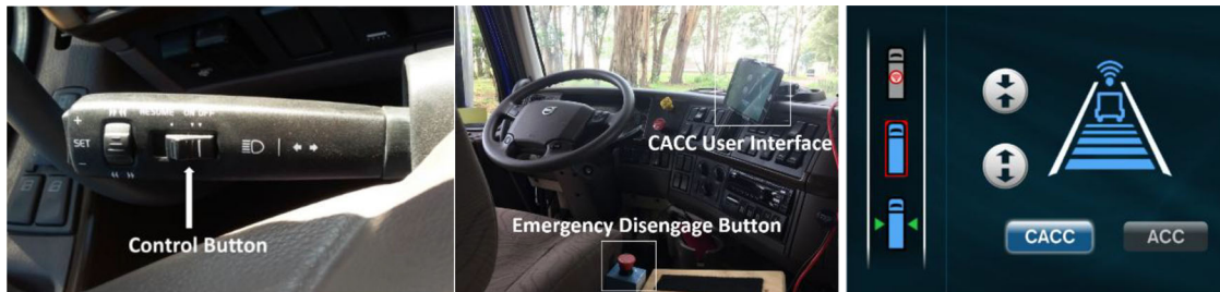
Figure 2. The CACC control stalk (left), truck cabin interior with the CACC user interface and emergency disengage button (middle), and the CACC user interface layout (right).
